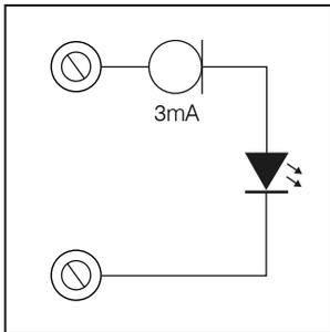
The trigger input circuit for **VCT, VTS & VTR** products is shown below:
